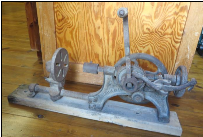
A vintage hand-cranked Drill Press (would have been mounted vertically), was donated by Ilta Hall. An embossed label reads "Triumph 71".
