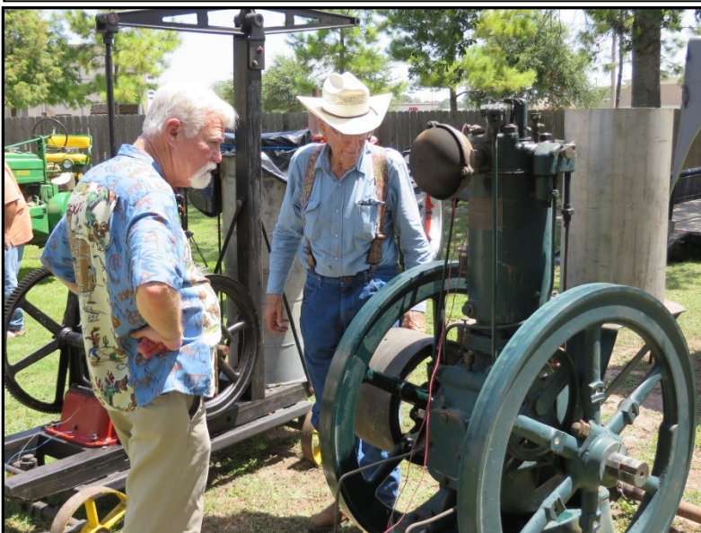
Jay Warren (left) looks at the restored “hit & miss engine” that used to run the Grist Mill located in the Cypress Top Park today. Gerald Lowery (right) of the Sharecroppers Early Engines and Tractor club demonstrates how it works.
